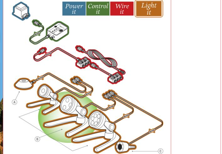
**Includes 12V quick-connect, weatherproof electrical connection. Used only with UL Listed Adapter Class 2 output. Outdoor use Max. Rated output 12 V ac, 5a 14.5' cord length.**
